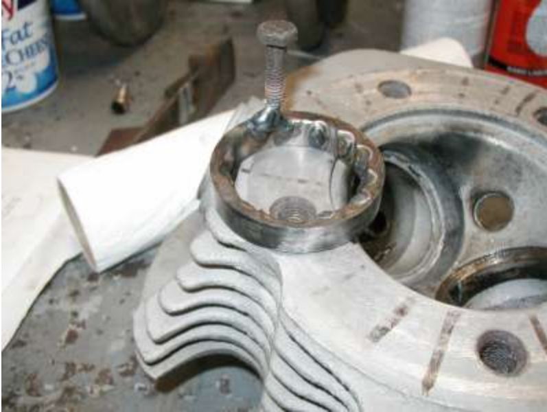
Pic 2 shows seat with bolt after removal.
