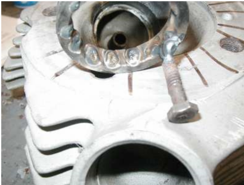
Pic 1 shows the seat with the numerous weld puddles top to bottom, also I attached a bolt to show how.
