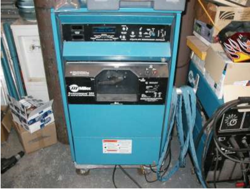
Pic 4 I have a secret weapon, Miller Intellitig 351 You can weld anything and I do, Chrome-moly, Al, Magnesium, Titanium, etc.
