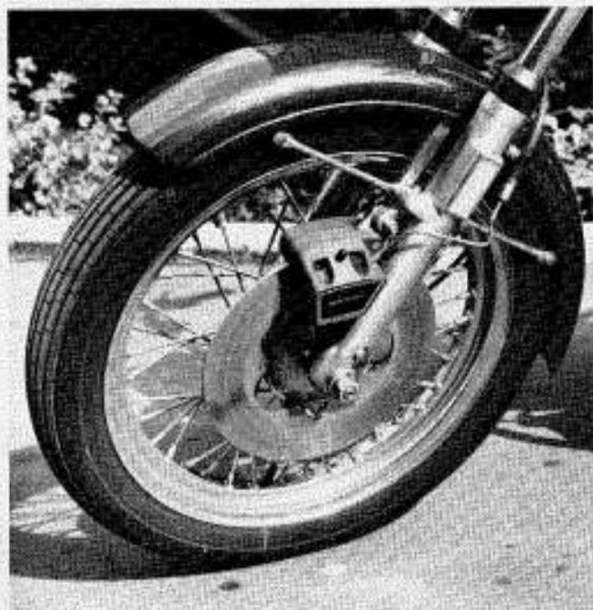
The front disc is sensitive up to a sudden and generally unexpected lockup.
