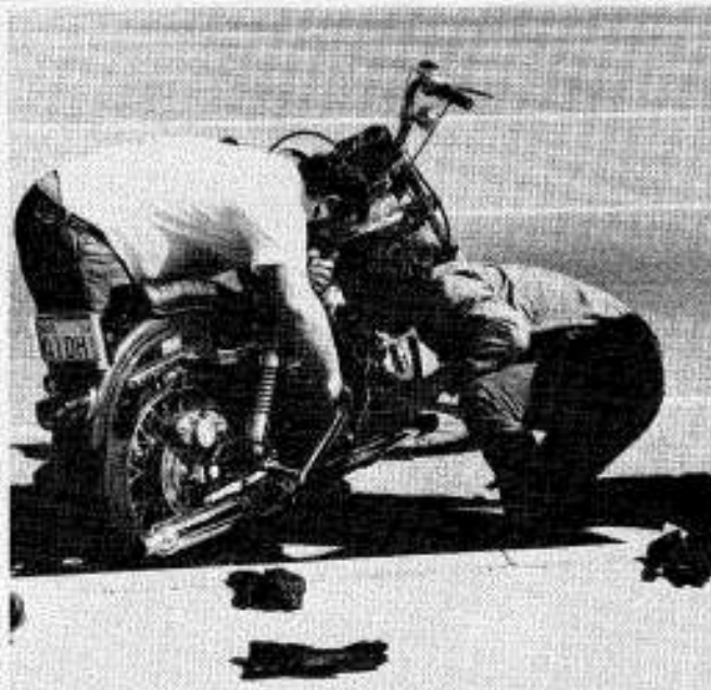
Teething problems on the electric start glide — eventually tracked to a non-factory-locked locknut on the clutch.
