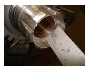
Ready to install the 2 new seals inside the end of the fourth gear: remember always clean /prime and put green Loctite on both the 2 small seals.
