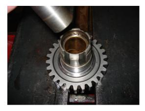
When the old bushing is out, I start by making a new one out of continuous cast bronze 660. Why making a new one? Often new bushings that came from different companies do not have enough material to clear everything, most of them, not to say all, are set at the factory to have minimal material to remove with a reamer, and often end up with many spots of material not removed.
