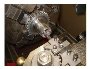
After the inside of the bushing is machined, I still continue modifying the end of the gear, here what I do, machining the recess a little bit deeper so I can put 2 seals in the end of the fourth gear instead of only one as OEM, the machining is done with either carbide or ceramic insert (much easier with a ceramic insert), the total depth required is 7/16 inch, instead of the 3/16 OEM, you can see the small oil groove inside the bushing not too deep but just enough to lubricate.
