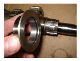
You could see the spacer with the oring inside ready to be slip on the OEM gear, just put very small amount of grease around the o-ring to avoid scraping it.
