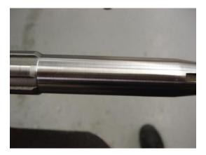
When everything is properly done, I set up the gear in the four jaws chuck and carefully dialing it to achieve a perfect run out, you have to be sure that where the bearing runs on, run perfect with a dial indicator.
