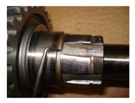
And the picture of the new spacer to accommodate the old gear.
