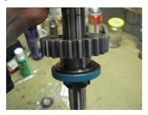
Here is the finished job with everything installed and ready to put the sprocket on. You could not see anything different from the outside, but this will definitely solve your leaking problem.
