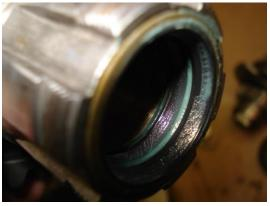
. When you are done with the gear, it is time to take care of the spacer, since the other main problem occur when some of the oil escape between the spacer and the shoulder of the gear, I always make a new type of spacer out of C1144 steel, with o ring groove inside so there is no way oil could escape.
