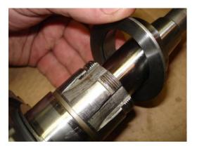
When everything is reassemble you will notice that there is now two seals at the end of the fourth gears including machining from all around the bushing with close tolerance and a 100% mating between both parts,100% mating between both parts means it will now take more time to wear out, if properly lubricate,... you will also end up with an O ring in the spacer....so no more silicone from the outside around the spline.
