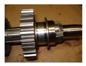
The first problem I have found is that the bushing is often too loose on the main shaft. So the first thing to do is press out the old bushing.
