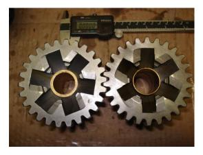
You will have to slightly polish the main shaft to get rid of small imperfection, or use a new shaft if it is too bad..., and then measure carefully so you could machine the bushing to achieve minimum clearance, in this case shaft measurement is .999 inch.
